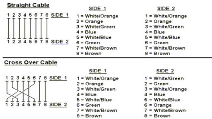
Figure A-1: Straight-Through and Crossover Cable
